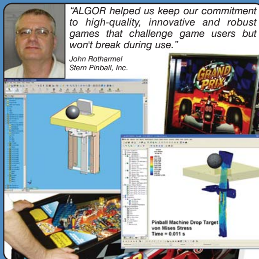
John Rotharmel of Stern Pinball modeled a pinball and plastic drop-target assembly in SolidWorks (upper left) and used ALGOR Mechanical Event Simulation to analyze the action of the pinball striking the drop target (lower right). The ALGOR results confirmed that the part needed strengthened before use in a new pinball machine.
