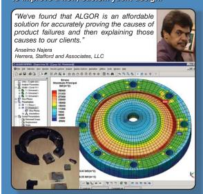
Herrera, Stafford and Associates, LLC studied a compressor head cover using linear static stress analysis and laboratory tests to discover the root cause of its failure.
