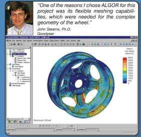
Goodyear engineers performed a linear static stress analysis on this aluminum automobile wheel, modeled in Pro/ENGINEER, in order to verify that safe stress levels were maintained in the wheel at zero inflation pressure for a new "run-flat" tire design.
