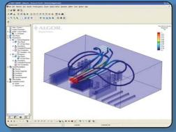
Steady fluid flow analysis was used to determine the velocity profile for fan-generated air flow within this electronic enclosure. Streamlines show the flow path over objects attached to the base.
