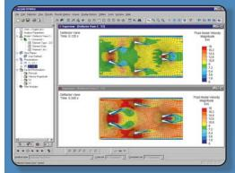
This unsteady fluid flow analysis shows the air flow patterns for this chamber, in order to study flow mixing. Since laminar flow was most desirable, the orientation of the vanes with respect to the inlet was critical.
