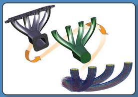
An exhaust manifold was modeled in KeyCreator (left); after specifying the surfaces for modeling the fluid medium in FEMPRO, a new part was automatically created (middle) where a steady fluid flow analysis was performed to determine velocity magnitude results (bottom right).
