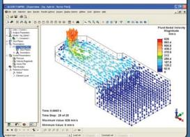
The Hewlett-Packard Company optimized ink flow in the ink feed channel of this thermal inkjet print head with unsteady fluid flow analysis to maximize print quality.
