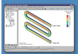
A steady fluid flow analysis was performed on an aluminum heat exchanger to calculate velocities for determining the effect of forced convection on the temperature profile.
