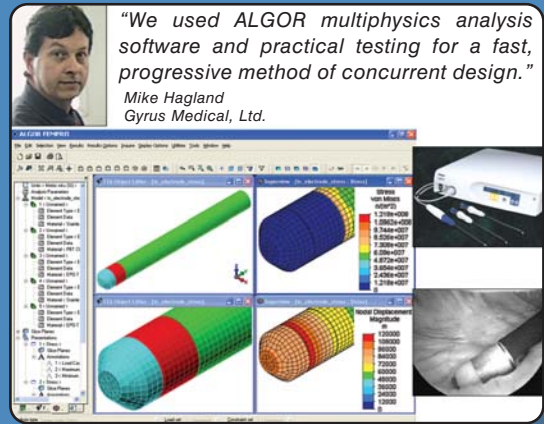
Engineers at Gyrus Medical, Ltd. used multiphysics software to determine the temperature and thermal stress distribution for this temperature control electrode, which heats soft tissue during arthroscopic surgical procedures.
